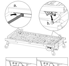
In the head end, slide the lifting mechanism gliding blocks into the guideways on the mattress support platform and in the foot end lower the mattress support platform onto the lifting mechanism until it engages with an audible click.
