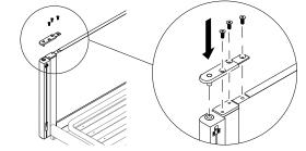
Fix the pillar and bed end board with the plate and the three screws.
