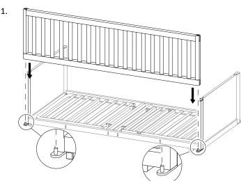
Place the side rail onto the pins on the bed end frames.
