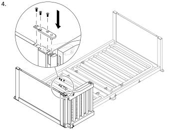
Fix the side rail and bed end boards with the plate and the three screws.
