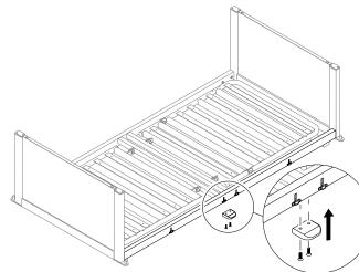
Fix the center wedge with two screws to the underside of lateral square tube of the mattress support platform.
