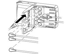
Plug in the cables of the mattress section actuators and close the lid of the control unit.
