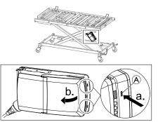
Press in the two latches (A) on the control unit with a pointed object (e.g. screwdriver) and open the lid.
