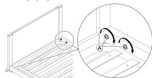
Completely tighten screws A in each corner of the bed.
