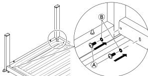
On both sides of the bed insert the screws (A) with their washers (B) and tighten them until the bed end frame is stable but till slightly adjustable in angle.
