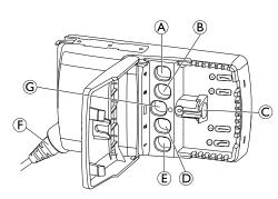
The actuator sockets inside the control unit are labeled with symbols and colors, indicating where to connect the respective plugs.
