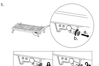
On both sides of the mattress support platform pull the red locking pin and turn it 45° clockwise to engage it in the unlocked position.
