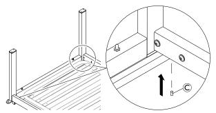
Position the bed end frame at an 90° angle to the mattress support platform and on both sides of the bed insert the grub screw  $\mathbb{C}$  until feeling a resistance.
