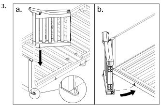
Place the side rail onto the pin on the bed end frame and close it , so it engages to the lateral square tube of the mattress support platform with an audible click.
