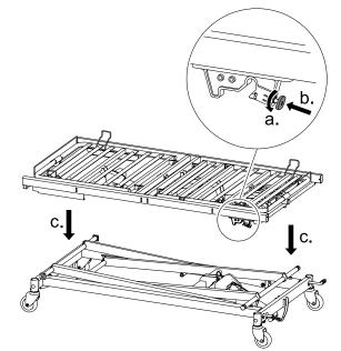
On both sides of the mattress support platform turn the red locking pin by 45° counter-clockwise and let it engage in its locked position before lowering the mattress support platform onto the lifting mechanism.
