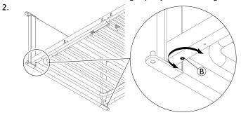
If required use the grub screws (B) to adjust the angle of the bed end frames until the side rails fit and function properly.
