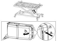
Press in the two latches (A) on the control unit with a pointed object (e.g. screwdriver) and open the lid.
