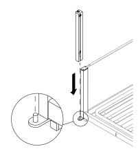
Place the pillar onto the pin on the bed end frames with the guideway facing towards the other end of the bed.
