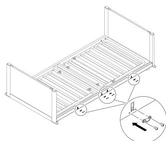
Fix a small wedge with two screws below each of the four slots on the lateral square tube of the mattress support platform.
