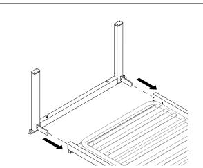
Insert the connectors of the bed end frame into the lateral square tubes of the mattress support platform.
