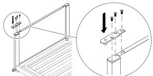
On one side of the bed temporarily install the plate to fix the bed end board to the bed end frame until a side rail has been mounted in the other side of the bed.
