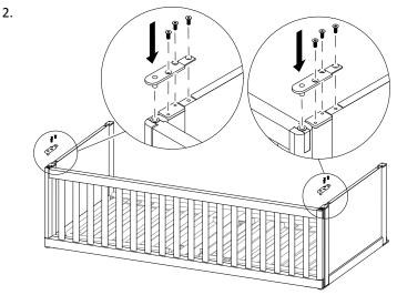
On both ends of the bed, fix the side rail and bed end boards with the plate and the three screws.
