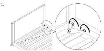
Slightly loosen screws (A) in each corner so the bed end frames are still stable but slightly adjustable in angle.
