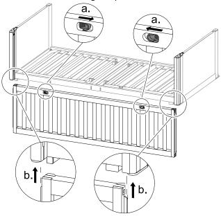
Push and hold the two latches towards each other and slide the side rail into the guideways of the pillars from below.
