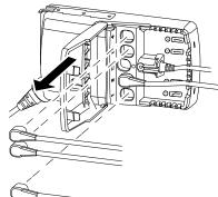
Unplug the cables of the mattress sections actuators from the control unit and close the lid of the control unit.
