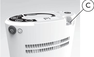
A close-up photograph of the nasal cannula outlet port, labeled 'C', on the side of the oxygen concentrator. The port is a circular socket with a cover.                                                 |
